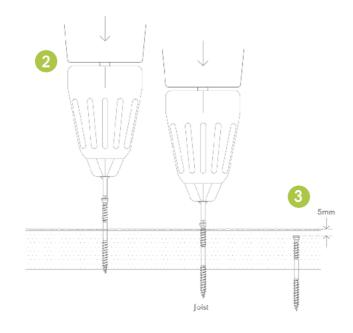
Failure to use our Durafix fixings with the bit provided or not fitting according to these guidelines may invalidate the warranty and affect the overall look of the deck. Two fixings per board should be used where the board crosses a joist, we advise to use three at the ends of the boards.
